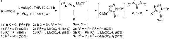
which the corresponding aryl azide was introduced into the reaction mixture, followed by the corresponding electrophile (Scheme 1). With this approach, no separation of intermediate products is required, and the resulting solutions of organomagnesium derivatives can be separated and used to synthesize several different chloro-, bromo-, and iodotriazoles 1–3. The method is demonstrated with 8 examples, all compounds were obtained with good yields.
